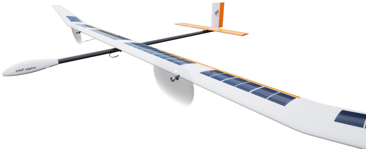
Figure 1: 3D rendering of the High Altitude Platform (HAP-alpha).
