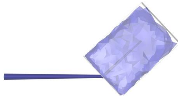
Figure 3 Automatic background mesh hole cutting
