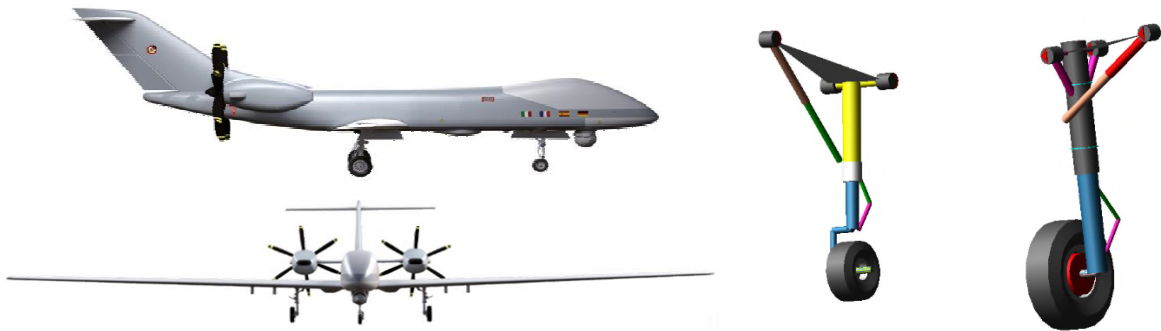
Figure 1: Eurodrone configuration (left) and the LEUAV NLG and port MLG MBS model (right)
