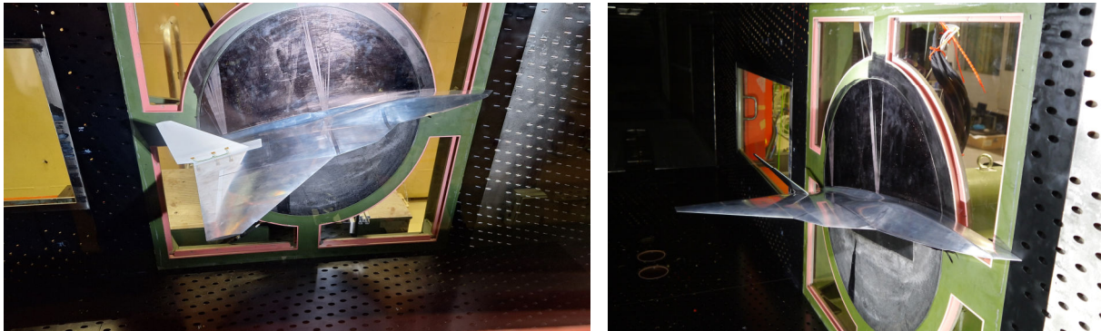
Figure 2: DLR-F23-T model mounted on the hydraulic-actuated pitching test rig in the perforated test section of the DNW-TWG wind tunnel.
