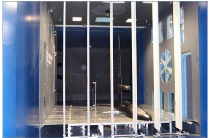
Figure 2 - GLA aero-servo-elastic wind tunnel model and installation in test room at PoliMi
