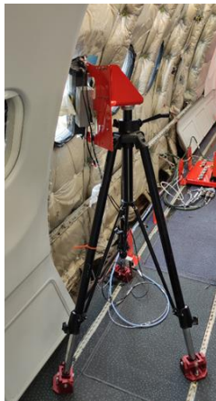
A. LiDAR system installed within the A330-MRTT fuselage.
