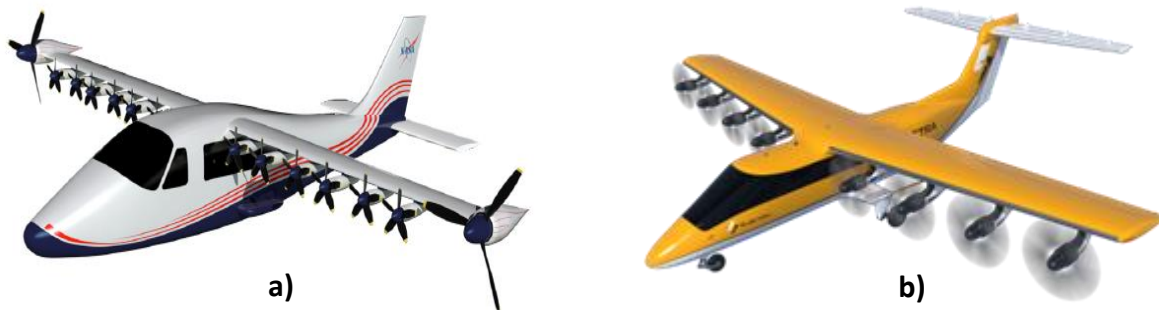
Figure 1: Novel aircraft configurations with Distributed Electric Propulsion. a) NASA X-57 Maxwell [7] and b) Electra EL9 eSTOL [8].
